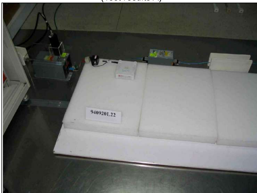
CS Test (Power line with CDN-M2) (Test results A)
