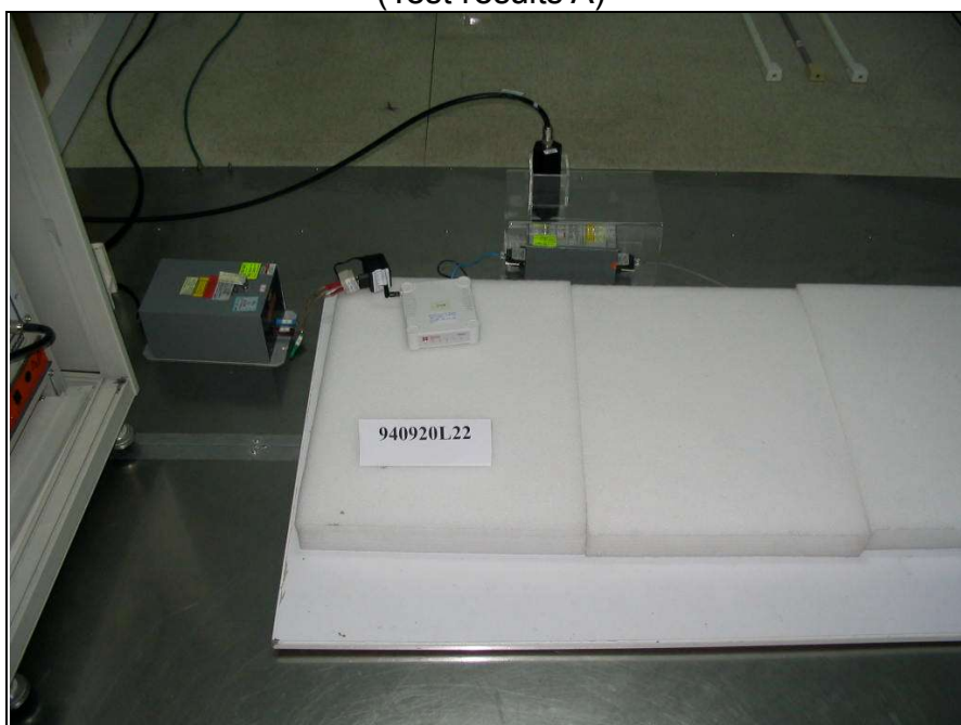
CS Test (RJ45 UTP cable with CDN-T8) (Test results A)
