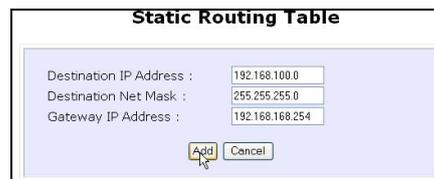
The screenshot shows the 'Static Routing Table' form with the input fields filled. The 'Destination IP Address' field contains '192.168.100.0', the 'Destination Net Mask' field contains '255.255.255.0', and the 'Gateway IP Address' field contains '192.168.168.254'. Below the fields are 'Add' and 'Cancel' buttons.
