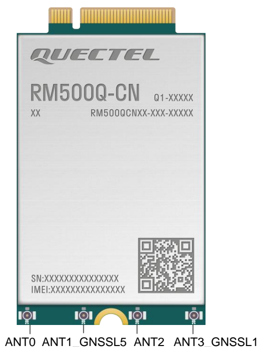
Figure 30: Antenna Connectors on RM500Q-CN
