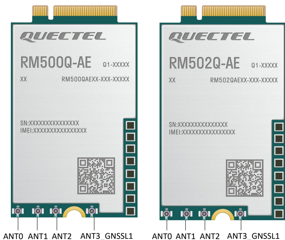
Figure 28: Antenna Connectors on RM500Q-AE & RM502Q-AE
