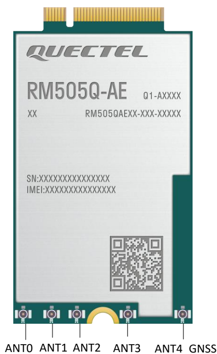
Figure 29: Antenna Connectors on RM505Q-AE
